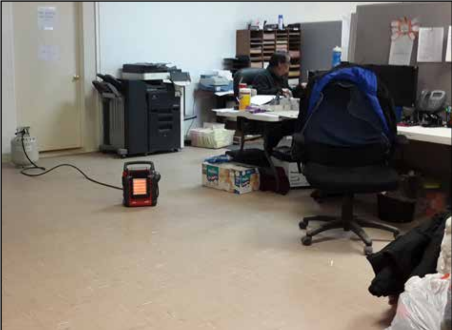
Employees work in unsafe conditions. Propane Heaters used for indoor heating and extension cords are lined up across the floors.
